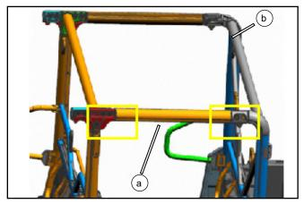
// Remove the seat (a) from the vehicle body (b).
