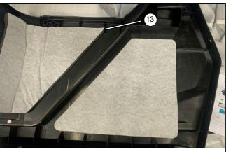
Paste the seat side sound absorbing cushion 1 (13) on the inner side of the seat RH panel, and tear down the protective film. Sound absorbing cushion comes with gum on the back side.
