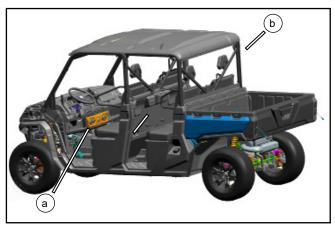
Remove the dashboard outlet panel (a) from the vehicle body (b).
