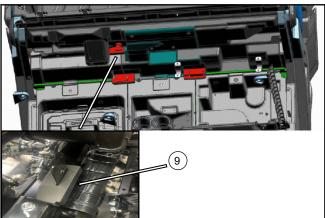
Install the fender front service cover plug (9) on the seat belt bracket.
