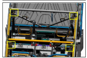
Remove all the bolts from the upper of the seat belt, and then remove the seat belt.
