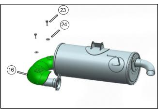
Secure the muffler pipe heat insulator (16) on the muffler exhaust pipe with bolts 6x16 (23) and washer (24).
