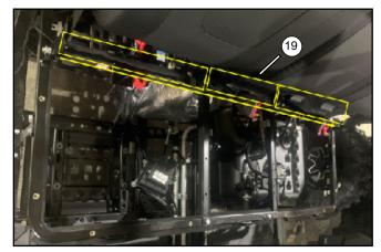
Paste the main seat middle lower fender tape (19) on the seat bracket as shown in the picture. Avoid the seat belt bracket. Cut and paste the tape according to the actual situation.
