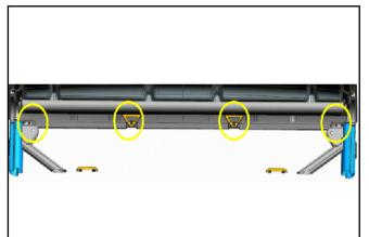
Remove four black bolts from the rear of the top roof.
