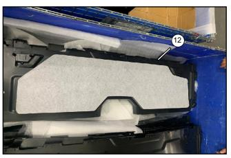
Paste the seat front sound absorbing cushion (12) on the inner side of the seat front lower panel, and tear down the protective film. Sound absorbing cushion comes with gum on the back side. (Paste on the rear seat for double-row vehicle)
