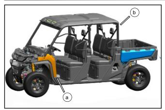
Remove the deco cover of driver & passenger side (a) from the vehicle body (b).
