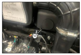
Install the seat rear fender plug (10) on the seat rear fender.
