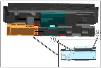
Install the fender front service cover insulator (11) on the fender front service cover with four self-tapping screws (25).
