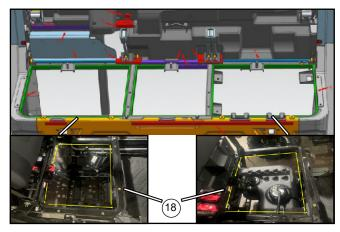
Paste the driver seat RH lower baffle tape (18) as shown in the direction of the arrow. When pasting, cut and splice the tape according to the actual length. The splicing gap should less than 3mm.
