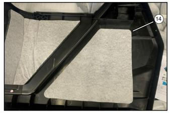
Paste the seat side sound absorbing cushion 2 (14) on the inner side of the seat RH panel, and tear down the protective film. Sound absorbing cushion comes with gum on the back side.
