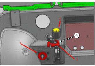
// Paste the turn plug (4) at the position as shown in the picture to ensure sealing.
