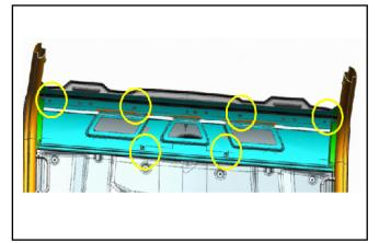
Remove six black bolts M6x16 from the front of the plastic top roof.
