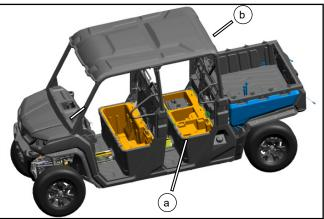
Remove the plastic component (a) under the seat and ECU plug from the vehicle body (b).
