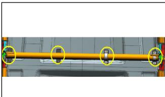
Remove eight black bolts and four top roof clamps from the middle cab assy.
