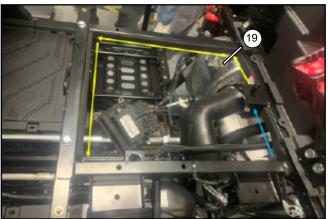
Paste the main seat middle lower fender tape (19) to the inner side of the seat bracket tube as shown in the direction of the arrow. Do not paste the side without the yellow arrow. Cut and paste the tape according to the actual situation.
