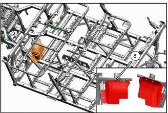
Secure the front heat insulator (8) on the frame with bolts 6x16 and washer.
