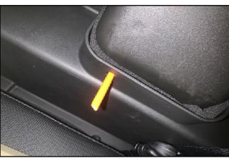
// Pierce the tape blocking the hole with an awl.
