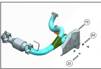
Secure the rear pipe heat insulator (15) on the rear pipe assy with bolts 6x16 (23) and washer (24).
