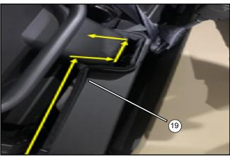
Take one half of the main seat middle lower fender tape (19) and paste it along the upper edge of the fender front service cover as shown in the picture.
