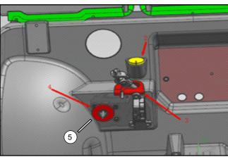
// Paste the brake plug (5) at the position as shown in the picture to ensure sealing.
