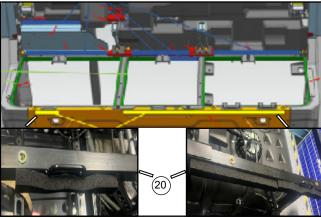
Paste the cab side tape (20) as shown in the picture. When pasting, cut and splice the tape according to the actual length. The splicing gap should less than 3mm.
