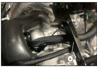
// Secure the clip of high-pressure oil pipe (a) to the hole of the seat bracket.
