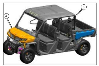
// Remove the cab cover (a) from the vehicle body (b).
