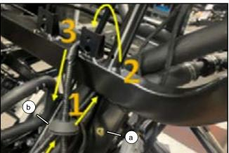
// In the front end of the heating cable, first hang the heating cable on the frame tube according to the direction of the yellow arrow as shown in the picture.
