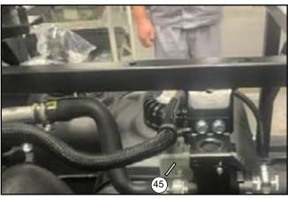
// Secure the heating pipe to the stop valve port with the clamp (45).
