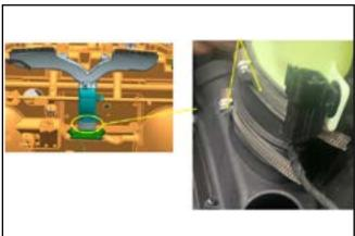
// Secure the bolt of the clamp with the fastening tool.
