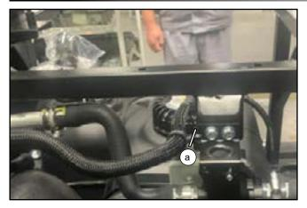
// Secure the clip of high-pressure oil pipe (a) to the hole of the stop valve bracket.
