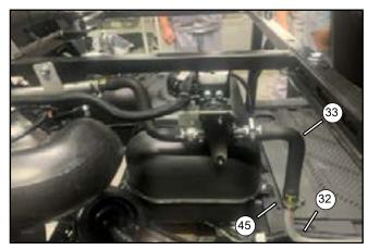
// Secure the clamp (45) on the air heater inlet pipe 4 (32) and connect it to the air heater inlet pipe (33), then use the fastening tool to tighten the bolt of the clamp.
